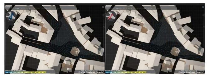
Figure. 10. Piazza Fontana Grande: Wind Flows Analysis. The analysis shows that, in the winter season (February threshold) there is an excessive ventilation in the North-South direction while, in the summer season (August threshold), a number of warm East-West flows are added (Source: M. Maretto).
